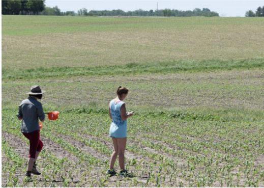
Figure 11. Global position systems (GPS) have changed soil sampling by improving pre-planning, re-use of sample data, and the accuracy of relating soil properties with covariates. The researchers in this photo created a sampling design using digital terrain analysis and are now locating those sample points using a GPS receiver.
